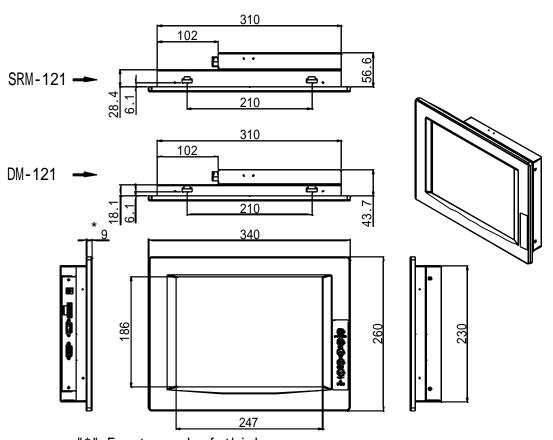
"\*" Front panel of thickness. By DM-121-AL / SRM-121-AL the thickness is 8 mm.
