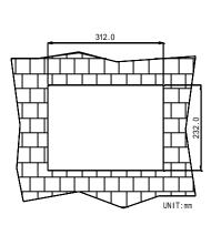
THE DIMENSION IS FOR PANEL MOUNTING (The flat panel thickness is 6mm or less than 6mm)
