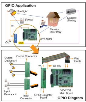
The connection points of each output device are common, normal open (NO), normal closed (NC)
